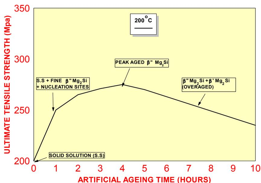
Figure 17: Typical ageing curve for 6000 series alloy.
