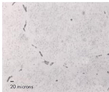
*Figure 9: Typical billet microstructure after induction preheating.*
