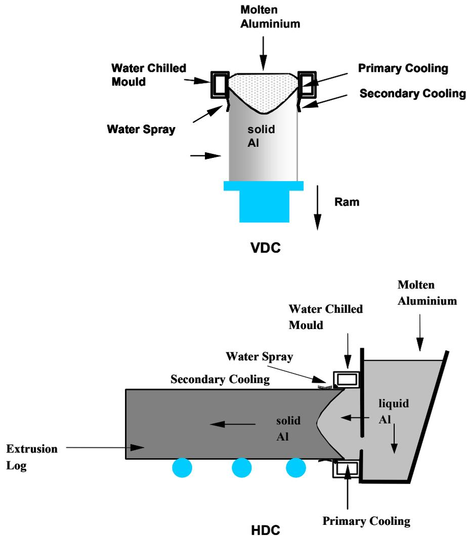
Figure 3: Schematics of VDC and HDC casting.
