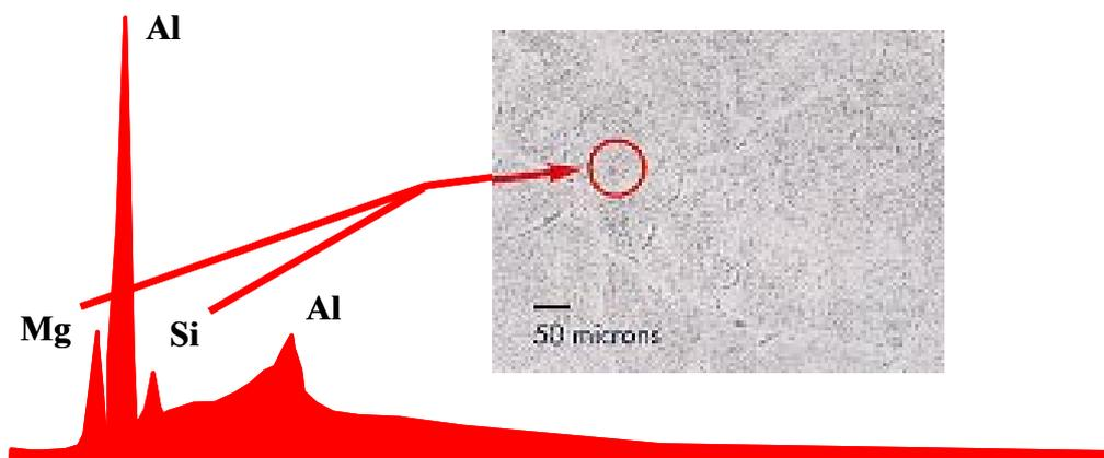
Figure 8: Micrograph of homogenised and cooled microstructure with energy dispersive spectrograph identifying the precipitated elements, (200 mag).
