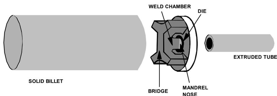
Hollow extrusions produced by these dies have longitudinal welds caused by metal flow around the supports for the mandrel nose or stub. The metal flows around the supports and is fused in the weld chamber before passing through the die.
