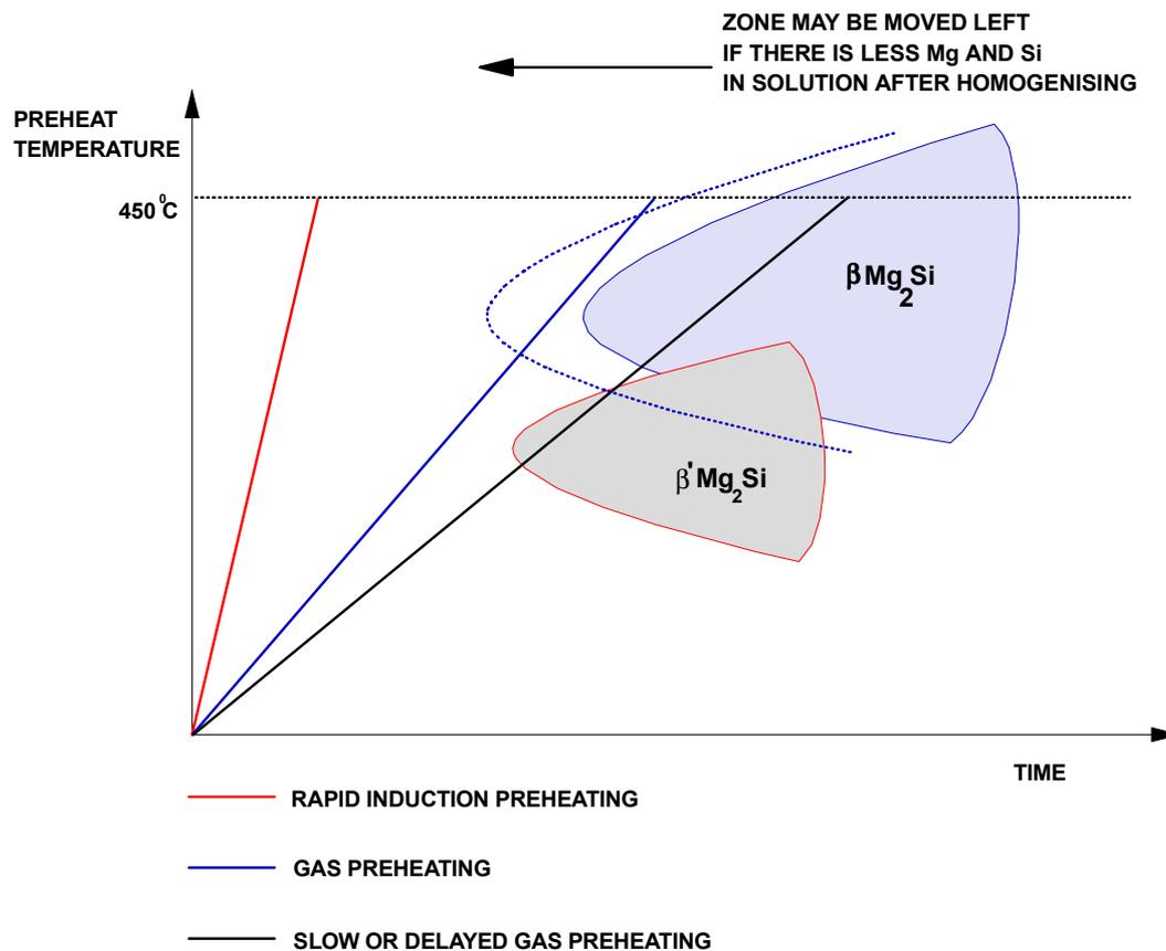
Figure 10. Graph of preheat rates and zones of  $\beta'$  and  $\beta$  Mg<sub>2</sub>Si formation.
