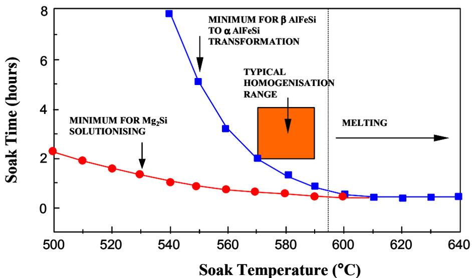
Figure 6: Homogenisation soak temperature versus time.
